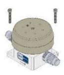
Attach Regulator to tool in predrilled and tapped holes for 3/8in (10mm) socket head cap screws.
