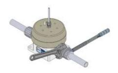
Torque liquid fittings to manufacturer spec. Use a backer wrench on fitting body.
