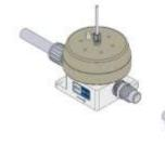
Loosely attach liquid connections. Ensure that liquid flows in the same direction as the arrow below the label. 6.
